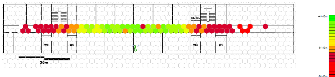
Figure 8: Coverage map of a single floor using a wifi AP placed inside a classroom.
